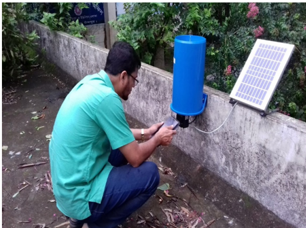
Recording of rainfall using handheld automatic rain gauges
